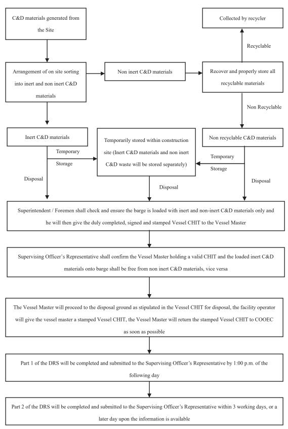
Procedure for dumping C&D materials by barge
