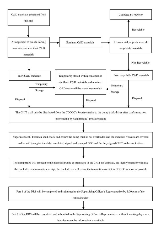
Procedure for dumping C&D materials by dump truck
