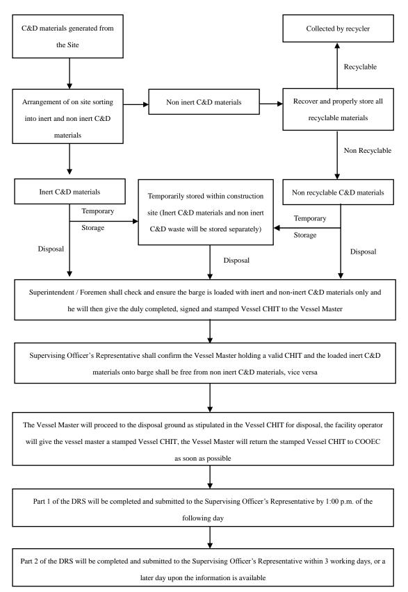
Procedure for dumping C&D materials by barge
